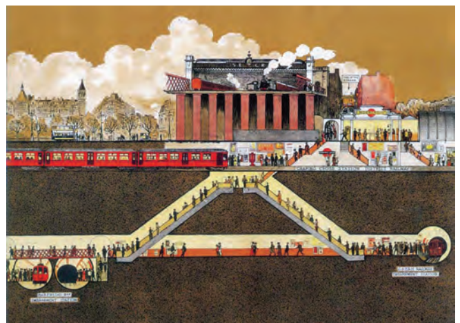
1914 cutaway of the underground lines at Embankment. To the left are the two Bakerloo line platforms and on the right the single Charing Cross, Euston and Hampstead (later Northern line) platform
